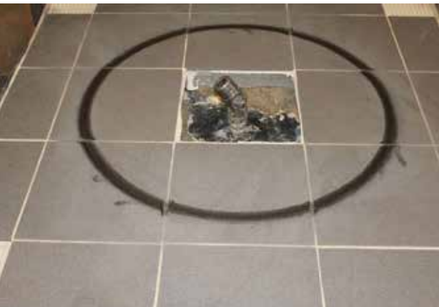
Fig 2. In the Robinson Floor Test, a weighted three-wheeled cart travels over a tile assembly in a 30-inch diameter circular path at a rate of 15 revolutions per minute for 30 to 60 minutes per cycle, for up to 14 cycles, with loads increasing from 300 to 900 pounds and wheel hardness increasing from soft rubber to hard rubber to steel from cycle to cycle. The assembly is assessed for damage after each cycle.
